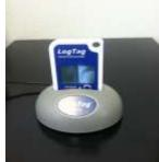
After downloading the data from the LogTag, review the data to determine what temperature was reached and the length of the excursion. Complete the **Temperature Excursion Checklist** (see below).
