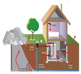
Radon gas rises up through the soil and is pulled into a house or building. It enters a home or building through cracks in the foundation, construction joints, gaps around service pipes or wires, and sump pits. It doesn't matter what type of foundation your home has—basement, crawl space, slab—your home could have high levels of radon.
