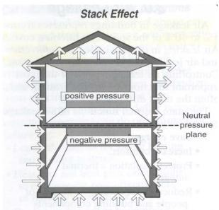
The stack effect is caused by the relative buoyancy of warmer air. Warmer air's upward force exerts an outward pressure. Airflow, through holes in the home's top, creates suction at lower levels, pulling air in. Arrows indicate the direction of positive pressure.
