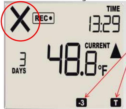
2. Press and hold the STOP button until "STOPPED" is displayed on the screen (approximately 2 seconds) and the REC symbol disappears. Release the button quickly.
